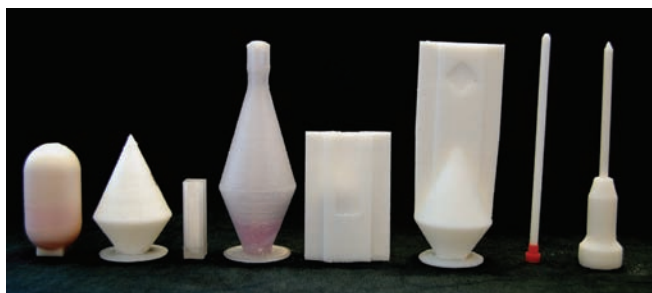
Fig. 1. 3D-Printed reaction flasks, cuvettes, and objects. From left: round-bottom flask made of ABS-N (F1), conical flask made of ABS-N (F2), UV cuvette made of ABS-K (F3), inert-gas flask with UV cuvette made of ABS-K (F4), IR cuvette made of ABS-N (F5), inert-gas flask with IR cuvette made of ABS-N (F6), NMR tube made of ABS-N (F7), and inert-gas flask/spinner with NMR tube made of ABS-N (F8).
